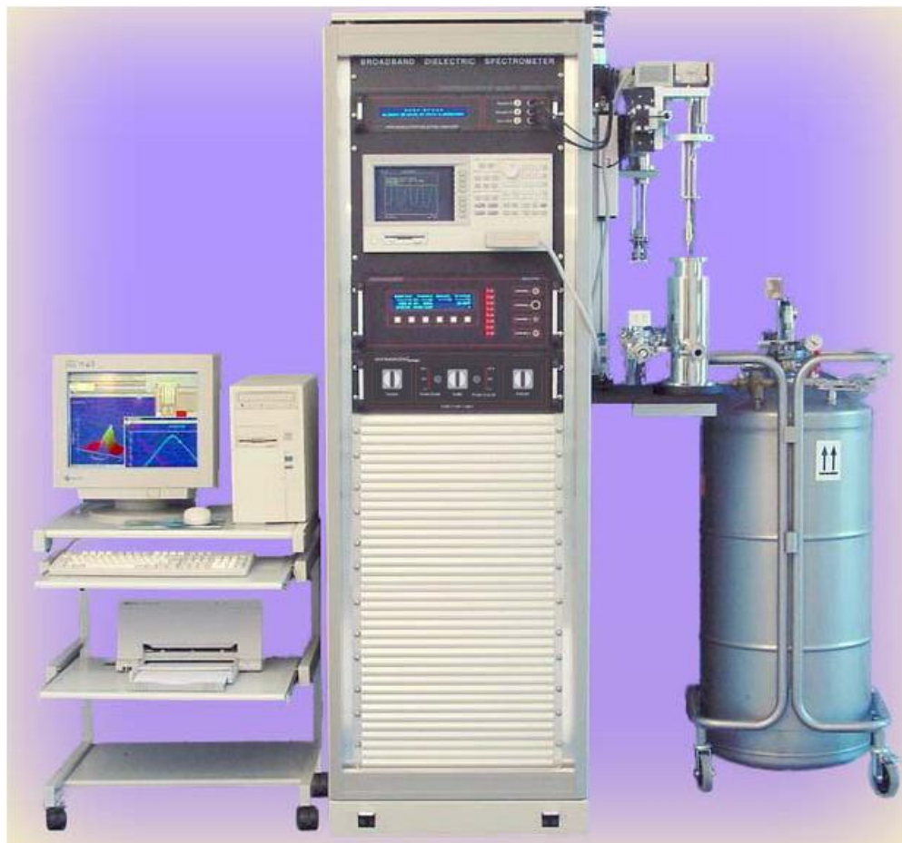
Figure 2.7 BES measuring system including the analyzer, temperature control system, the cryostat and sample holder cell, vacuum pump (hidden) and electronic data management.
