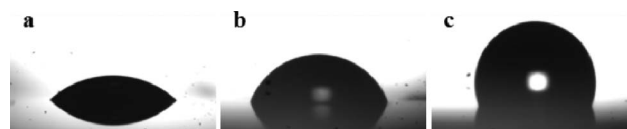
Fig. 2 Profiles of water droplets deposited on ThR surfaces: a) PTS-treated; b) untreated; c) OTS-treated.
