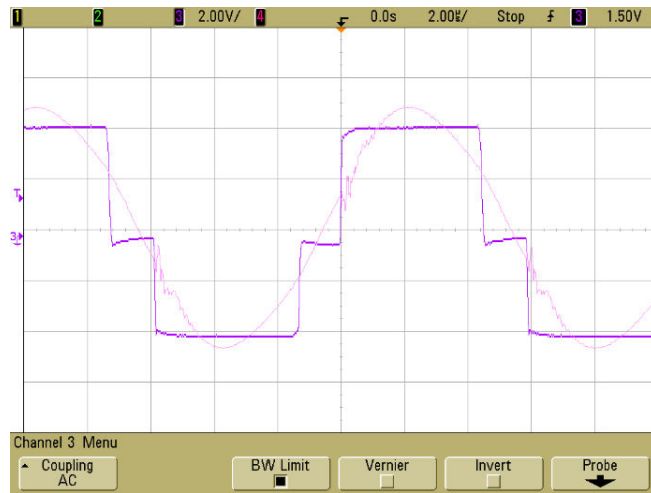
Fig. 8.11. Voltage and current of the transmitter coil
