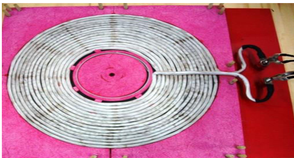
Fig. 8.1. Spiral coil-coupling setup with I core.
