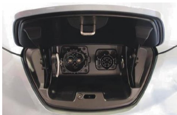
Figure 12.15. The standard J1772 receptacle (right) can receive charge from Level 1 or Level 2 equipment. The CHAdeMO DC fast charge receptacle (left) uses a different type of connector.
