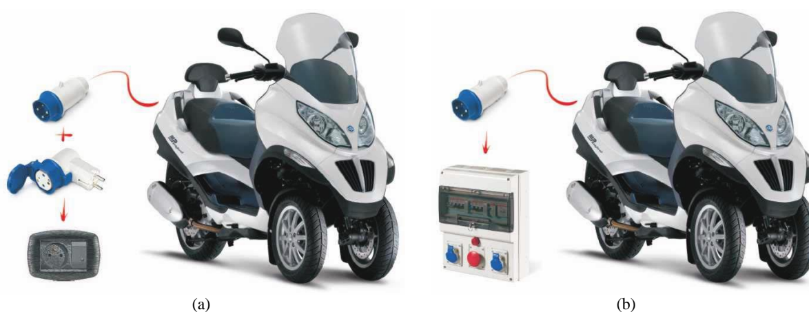
Figure 12.11. Type 3A connectors; a) Mode 1: charging in domestic environment (closed to third parties), b) Mode 3: charging in public areas (open to third parties)
