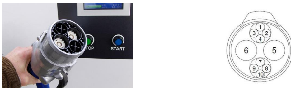
Figure 12.14. CHAdeMO pin layout and circuit diagram
