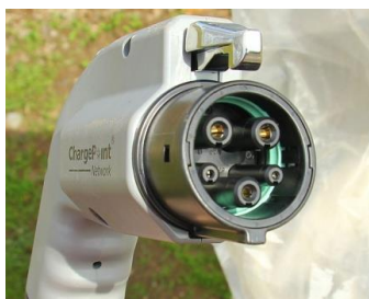
Figure 12.7. SAE J1772 – 2009 plug (Type 1) and its circuit diagram.
