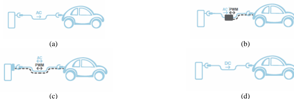
Figure 12.5. IEC 61851-1 four charging modes; a) Mode 1, b) Mode 2, c) Mode 3, and d) Mode 4
