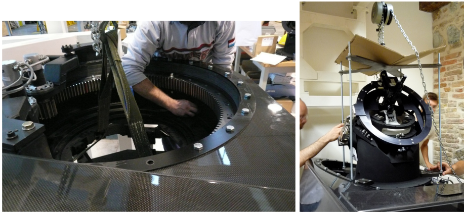
Figure 6.3: Left : GWS lower part fixing operation. Right : PR-I positioning on the carbon fiber arm.
