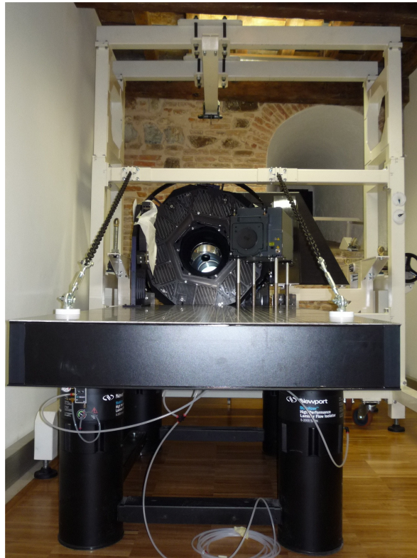
Figure 6.10: The optical bench completely held by the handling. The legs of the bench are separated from the upper part.
