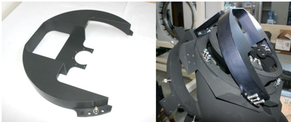
Figure 5.6: On the left, the flange holding the prime focus corrector, on the right the same flange already mounted on the pupil re-imager main structure.
