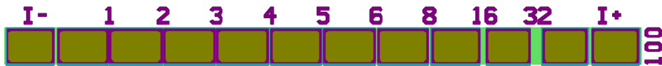
Figure 4.22: Wafer GO21-B mask layout of TLM structure; ohmic contacts are W \times D = 100 \times 130 \mu\text{m} .
