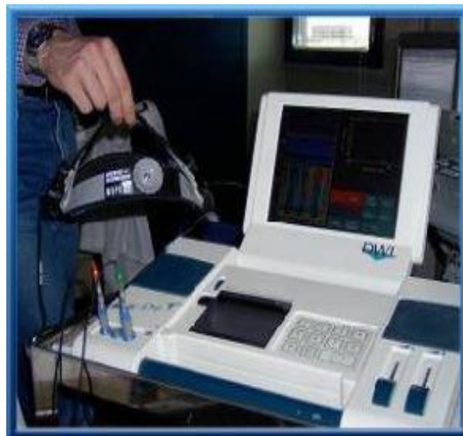
Figure 3.1 The transcranial Doppler apparatus (see also the Lam rack helmet; DWL/Compumedics, Singen Germany).
