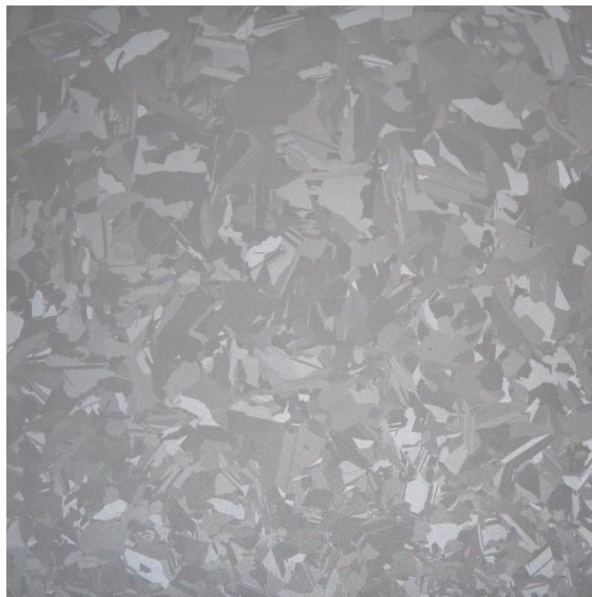
Figure 5.27 – Multi-crystalline silicon wafer obtained using the 450 kg iDSS furnace
