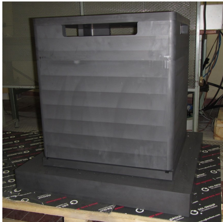
Figure 5.8 – Graphite susceptors in use in the 120 kg iDSS furnace built at University of Padova
