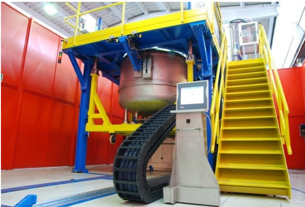
Figure 5.9 – 450 kg iDSS furnace
