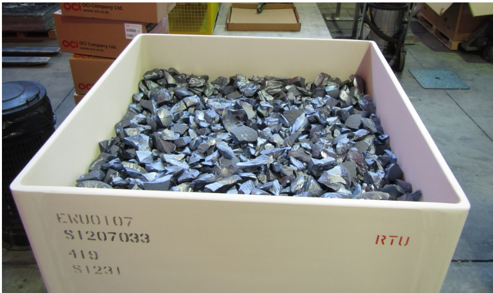
Figure 4.10 - 350 kg polysilicon charge in a quartz crucible used in an induction heating directional solidification furnace
