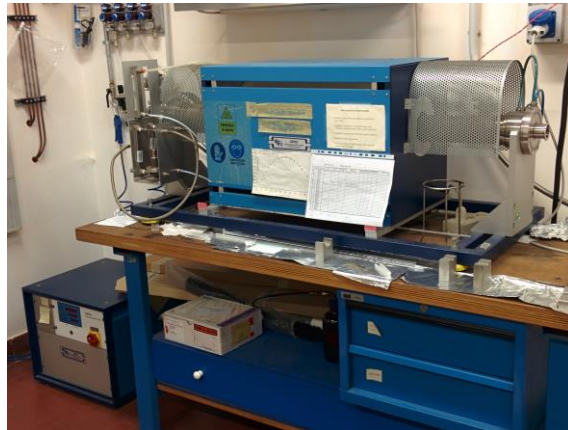
FIGURE 4 THE TUBULAR FURNACE GERO HOCHTEMPERATUROFEN GMBH (MODEL F-VS 100-500/13)
