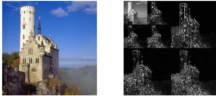
Figure 1.4: On the left, the well-known Lichtenstein image, considered a severe test bench for processing techniques. On the right, the result of a two level wavelet transform, comparable to the JPEG2000 compression format.
