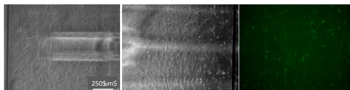
Figure 3.8: Human fibroblasts integrated in microfluidic chamber of Platform C.
