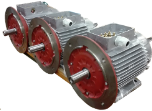
Figure 12.2: Motor prototypes manufactured for the study: one SyR machine and two PMASyR machines.
