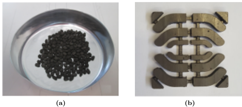
Figure 12.5: MQIP-M260 pellets used for the injection moulding (a) and final BMs samples (b).
