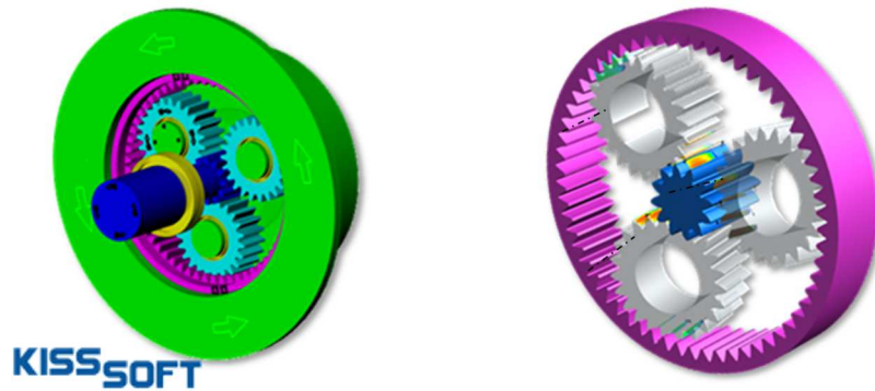
Figure 4.2 KISSsoft model of the planetary gear set located in the hub of an axle for agricultural vehicles.
