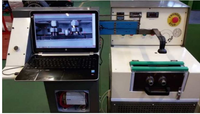
Figure 6.18 First concept of the vision system for the automatic inspection of the specimen's surface [143].
