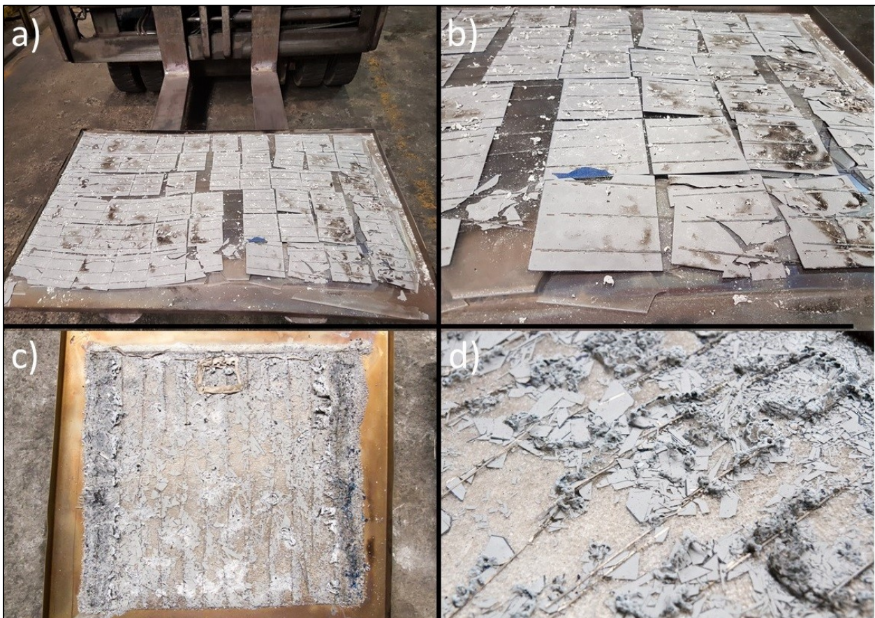
Fig. 4.32 Two PV panels after the heating treatment: a, b) panel that have unbroken glass before the treatment; c, d,) panel which have the glass already broken before the treatment.
