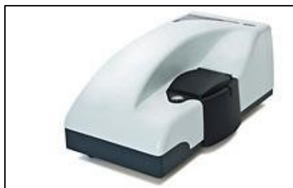
Fig. 2.10 Zetasizer Nano ZS used for laser diffraction.
