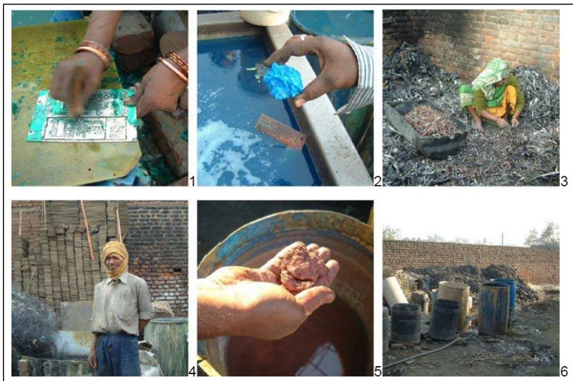
Fig. 1.8 The extraction of copper from printed wiring boards (PWB): (1) manually removing varnish, (2) recovering copper-sulphate after submerging PWBs for 12 h in sulfuric acid followed by boiling off H_2O using PWB residues as a fuel, (3) manually segregating the copper layer and glass fibers after burning multi-layer PWBs which are resistant to acid, (4) scrap iron is added to the remaining liquid to react with the dissolved copper, (5) fallen out copper slime is a third product bringing the total to 1 to 2 t of copper per month, (6) such an SME creates about 12 jobs, however at high external costs.
