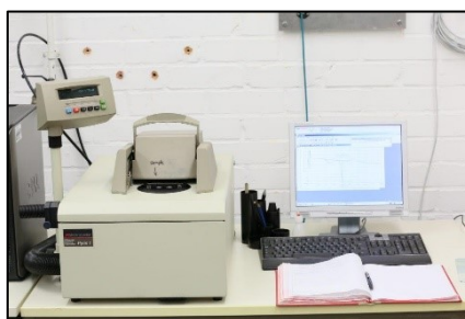
Fig. 2.14 Pyris 1 Thermobalance used for TGA analyses
