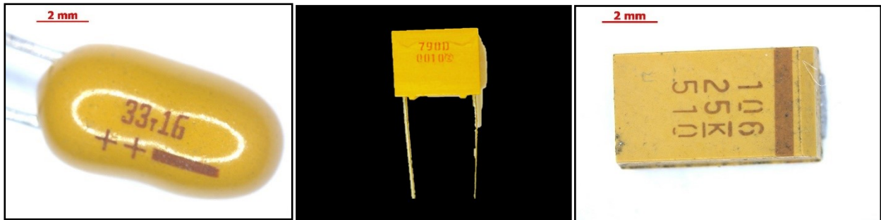
Fig. 5.4. The three type of tantalum capacitors analyzed.
