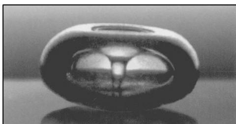
Fig. 1.30 Asymmetrical collapse of bubble at 25kHz [299].
