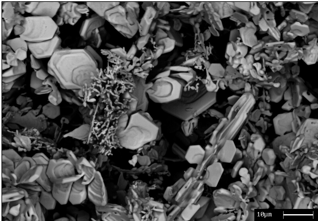
Fig. 4.41 SEM image of the deposit obtained by electrodeposition by a high acidity solution. It is interesting the particular hexagonal shape of silver crystals.
