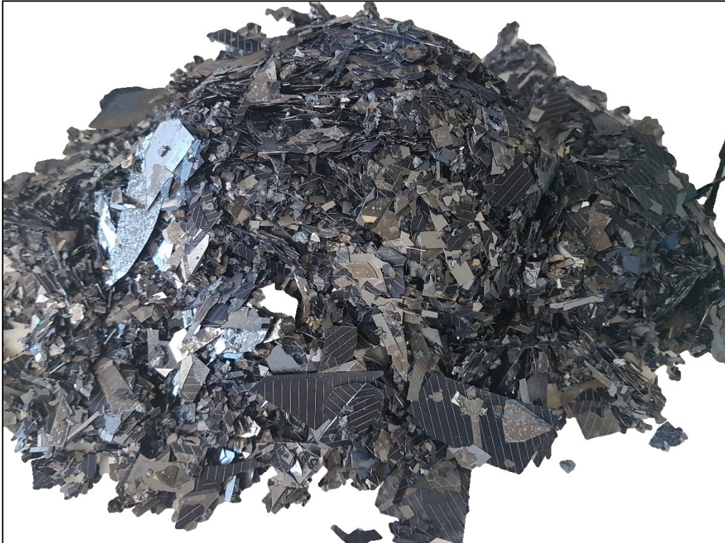
Fig. 4.39 The PV cells after the treatment with sodium hydroxide.
