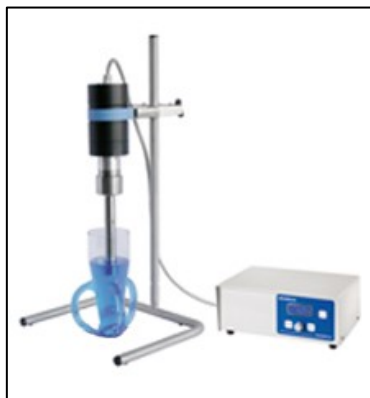
Fig. 2.8 Sonopuls HD 3200 used for ultrasound generation.
