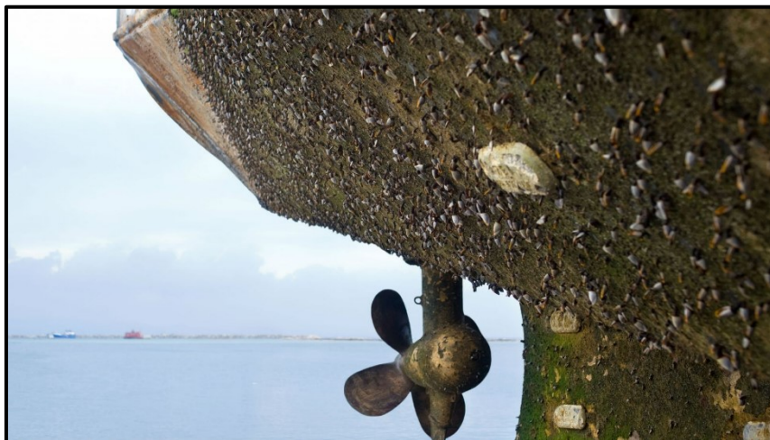
Fig. 7.16 Example of fouling colonization of a vessel [64].
