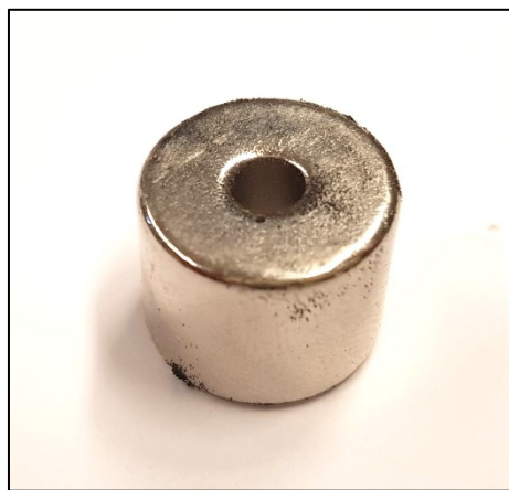
Fig. 5.15. The NdFeB magnet typically used in washing machine.
