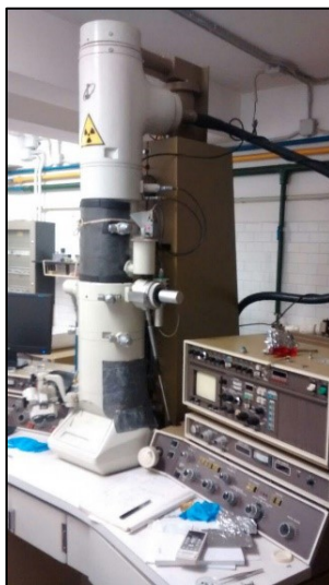
Fig. 2.9 JEOL 200CX used for TEM analyses.
