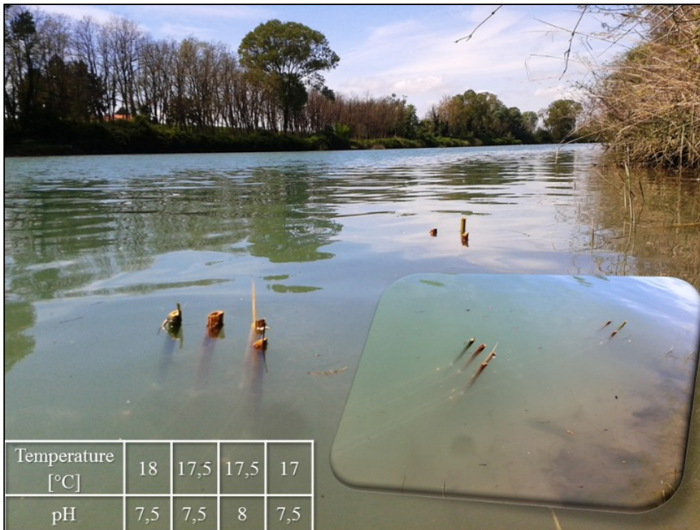
Fig. 7.18 Image of the place selected for the antifouling tests with the samples immersed in the estuarine water. In the table on the bottom left are reported the pH and temperature values recorded at the four sampling times.
