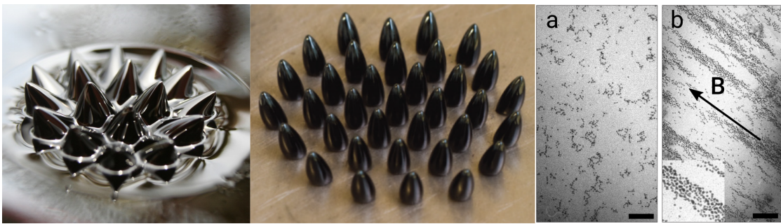
Figure 2 : (Left) Normal-field instability induced by a permanent magnet on a pool of ferrofluid. (Center) Self-assembly induced by a magnetic field taking advantage of the normal-field instability. The liquid has been deposited on a superhydrophobic surface [31]. (Right) a. Nanoparticles dispersed in the bulk of the ferrofluid in absence of the magnetic field. b. Chain-like aggregates in the bulk of the ferrofluid generated by the application of an external magnetic field [32].
