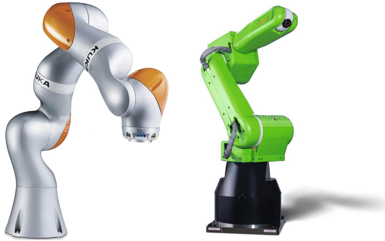
Figure 2: Collaborative robots: Kuka LBR iiwa (to the left) and Fanuc CR-35iA (to the right)
