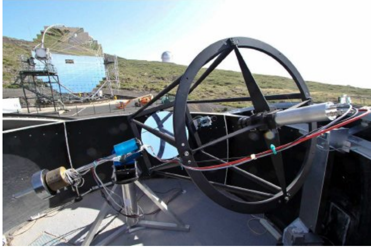
Figure 2.18: The LIDAR mounted on the roof of the MAGIC counting house.
