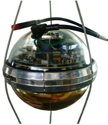
Figure 2.39: The digital optical modules of the IceCube detector.
