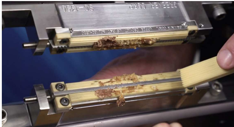
Figure 4: Residues accumulation on sealing jaws. [25]
