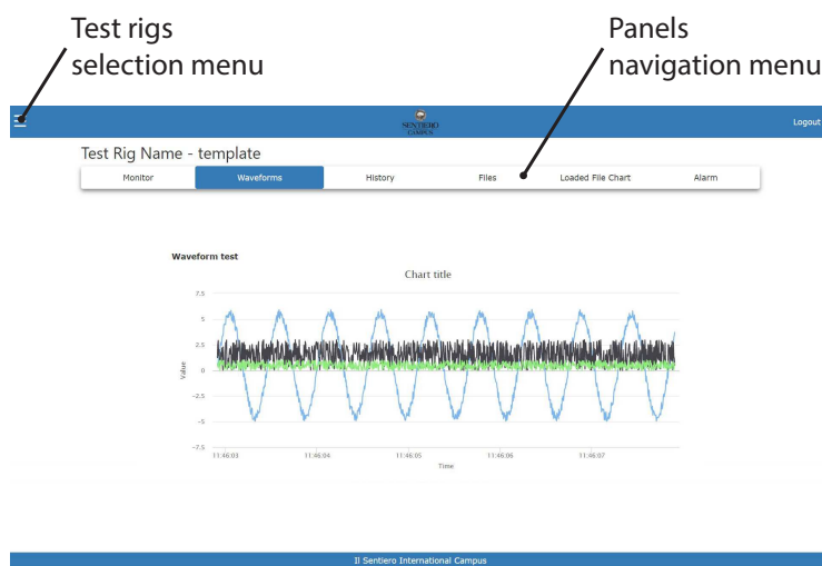
Figure 83: Example of dashboard developed for displaying data in real-time. It is possible to notice the panels relating to the display of historical trends, the selection of stored files and the graphing of their data and the alarm dashboard.
