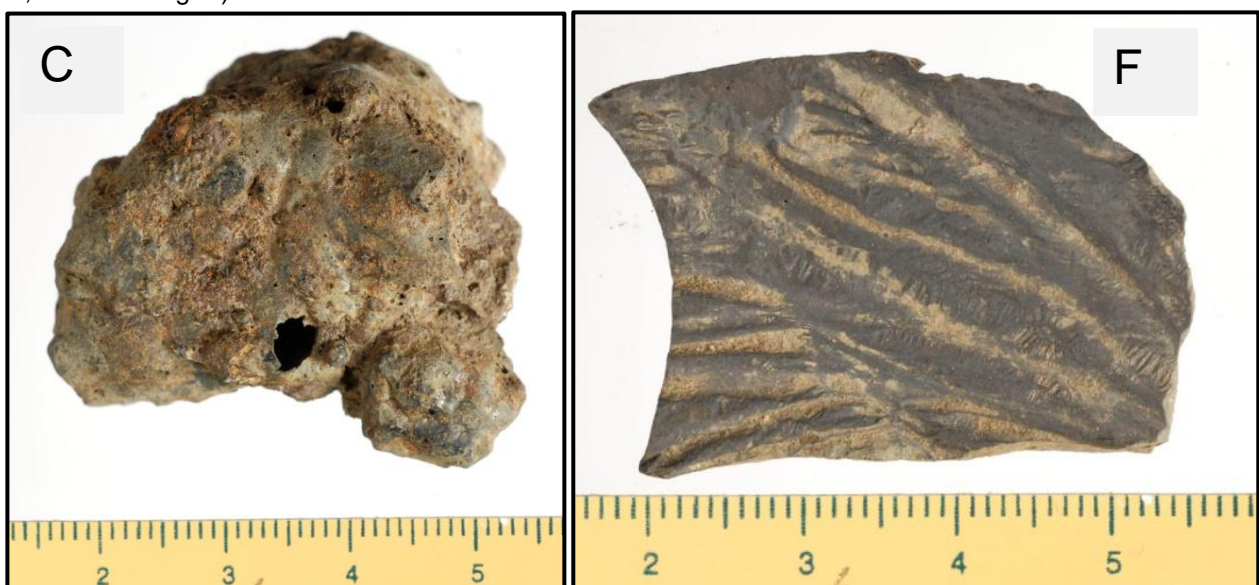
Fig. 4.2: Images of the two common types of slags founded in the LBA Alpine smelting sites (coarse slag: C, and flat slag: F)
