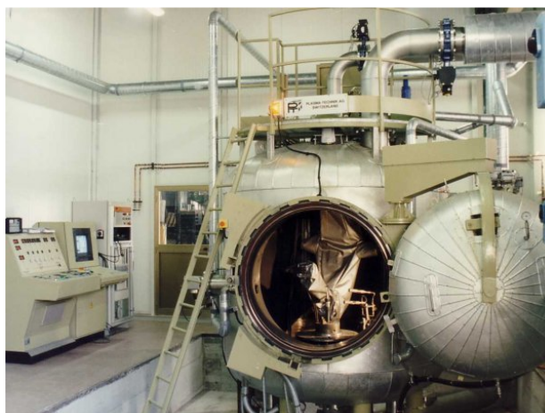
Figure 6.14: Controlled Atmosphere Plasma Spray facility at CSM (Centro Sviluppo Materiali), Rome.
