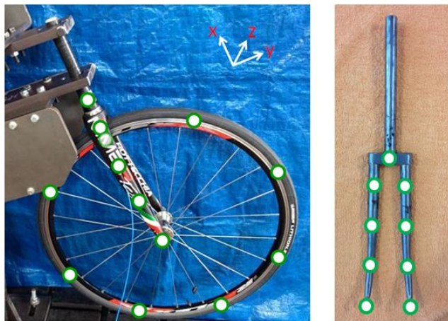
Figure 48 The tested front forks: carbon fork with the wheel (right) and steel fork (left).
