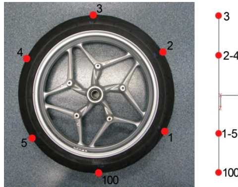
Figure 37 Measurement points for modal analysis.
