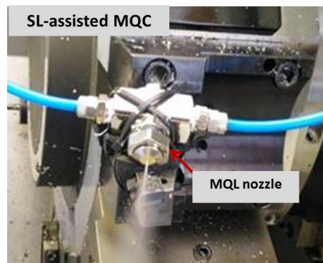
Figure 3.6. Experimental set-up for SL - assisted MQC technology.
