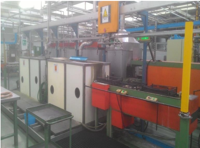
Fig. 8.5 - Static step annealing furnace used in the process
