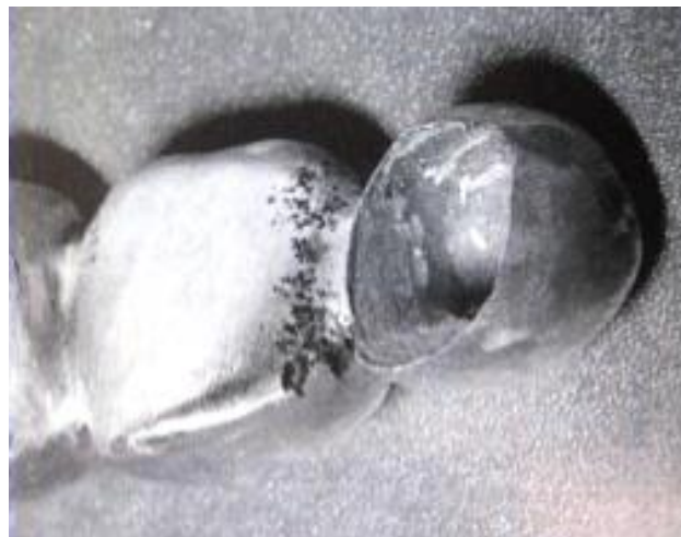
Fig. 4.5 - Shrinkage porosity defect in gold casting product
