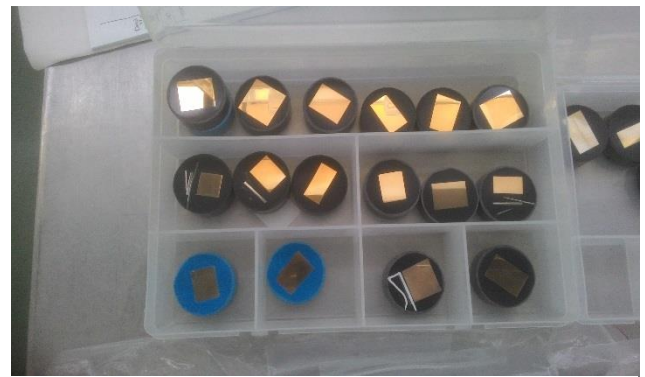
Fig. 5.2 – Samples of semi-finished products after metallographic preparation
