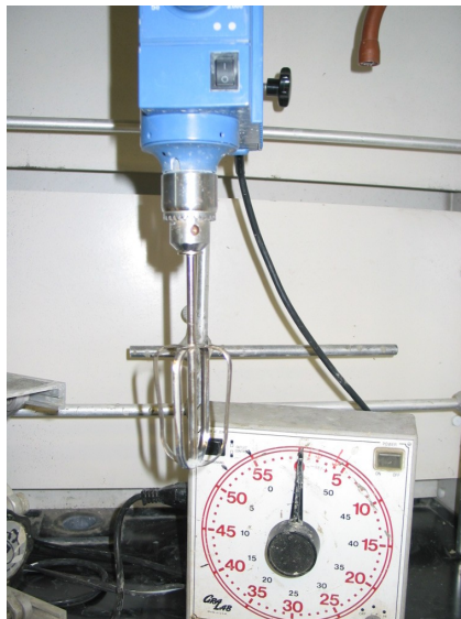
Figure 3.9: Eurostar mixer (power digi-visc, IKA Labotechnic) setup with hand mixer beater and timer connected to the mixer.
