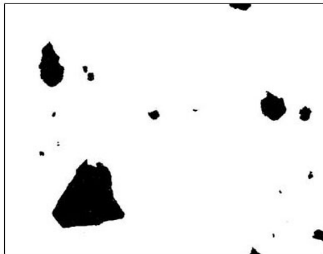
Figure 3. 26. Segmented images of the inclusions present in sample M101 with the corresponding frequency distribution diagrams: a) quartz inclusions; b) calcite inclusions; c) dolomite inclusions.
