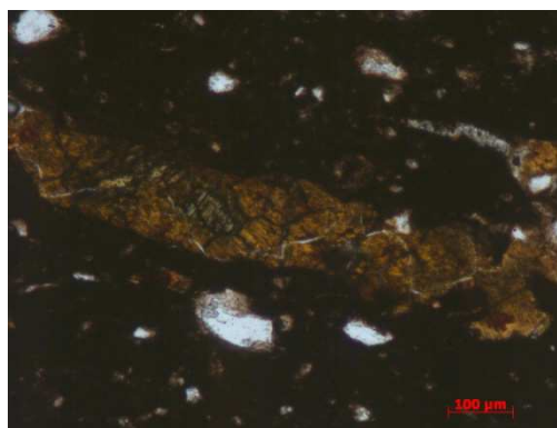
Figure 5. 1. Thin section photomicrographs of phosphate aggregate (P.1). The image was taken in crossed polars.
