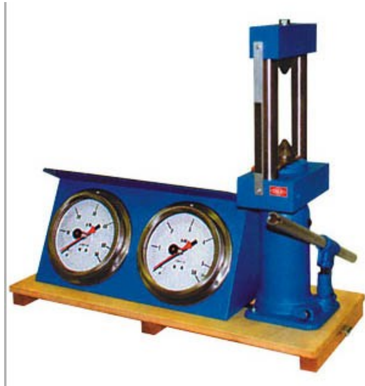
Figure 2.5: example of a point load test apparatus.
