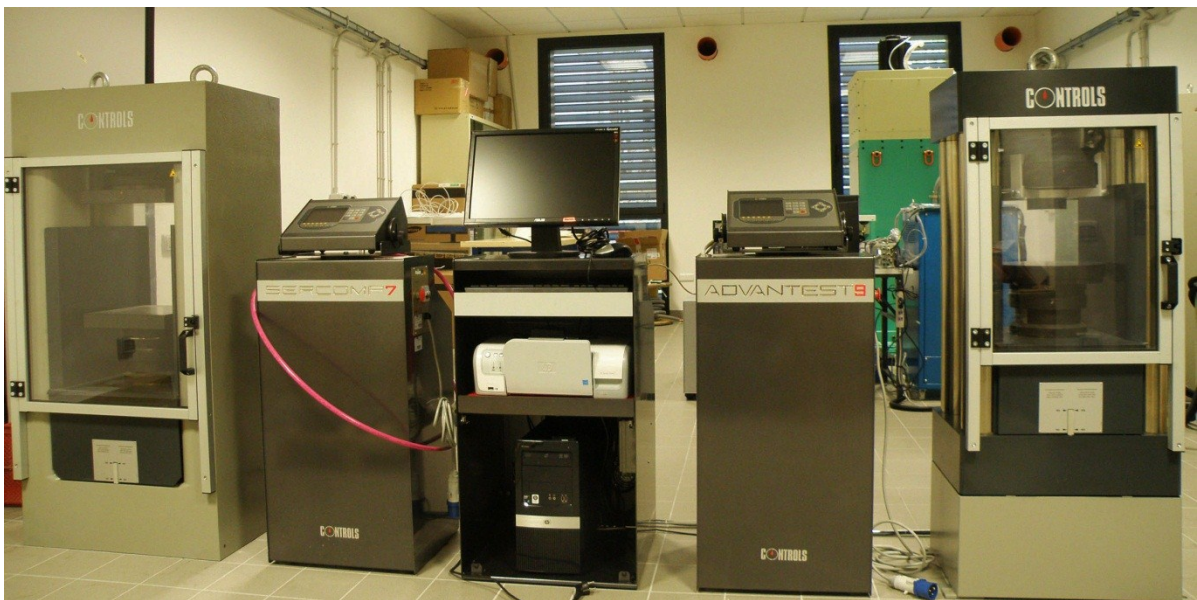
Figure 2.6: the automatic system ADVANTEST9 and SERCOMP7, available at the Rock Mechanics lab of the Geosciences department of the University of Padova (developed, produced and sold by Controls-Italia s.r.l.).
