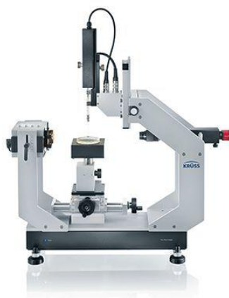
Figure 3.3. DSA 30S, the instrument used for contact angle measures.
