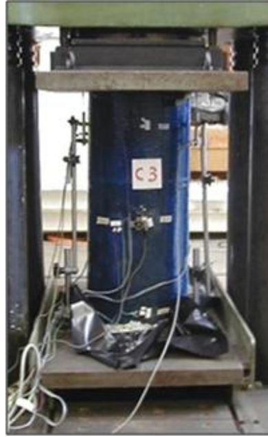
(b) Compression Test set-up for FRP-confined column
