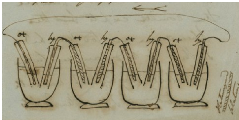
Figure 1.7 The first ever scheme of a fuel cell, drawn by Sir William Robert Grove in 1842. The original letter addressed to Michael Faraday is conserved at the Royal Institution in Mayfair, London.
