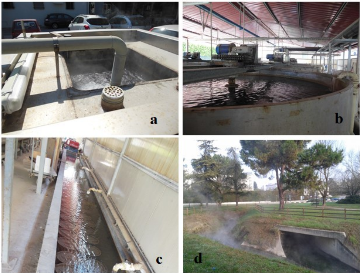
Figure 4.3 - (a) Thermal water well; (b) hot water pool for mud maturation with mechanical displacement of the clay; (c) hot water pool for mud maturation; (d) drainage system discharge into open canals.
