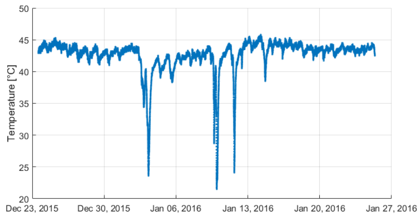
Figure 4.6 - Temperature in the drainage system of Abano Terme.
