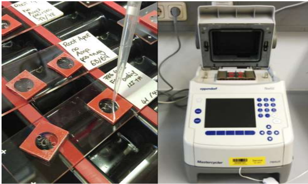
Figure 3.3. Approximately 50 µL of the DNase was added to each section through the hole of the hybridization chamber and covered RNase-free adhesive film. The slides were then incubated at 37 °C in the Thermoblocks or Thermal cyclers.
