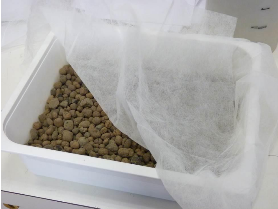
Figure 1. Each tray contains a 3 cm bed of expanded clay separated by a nonwoven fabric towel.
