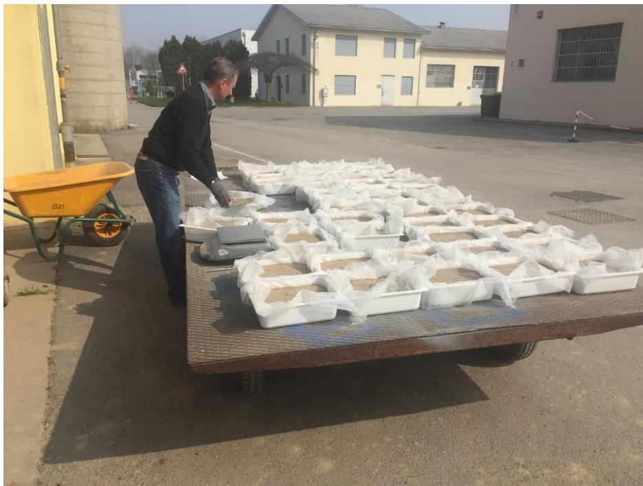
Figure 2. Weighing of the soil-sand mix (70% and 30% V/V) for each tray.
