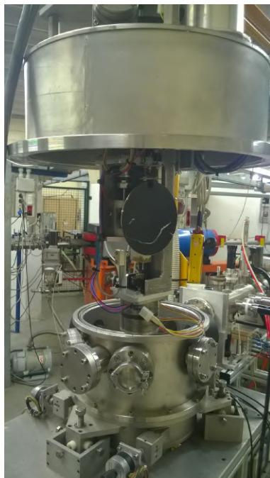
Figure 2.6. Measurement chamber with channeling goniometer at AN 2000 accelerator, 60 deg. beamline.
