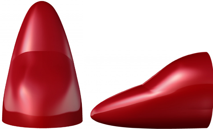
Figure 7.81: The final optimized nose geometry.
