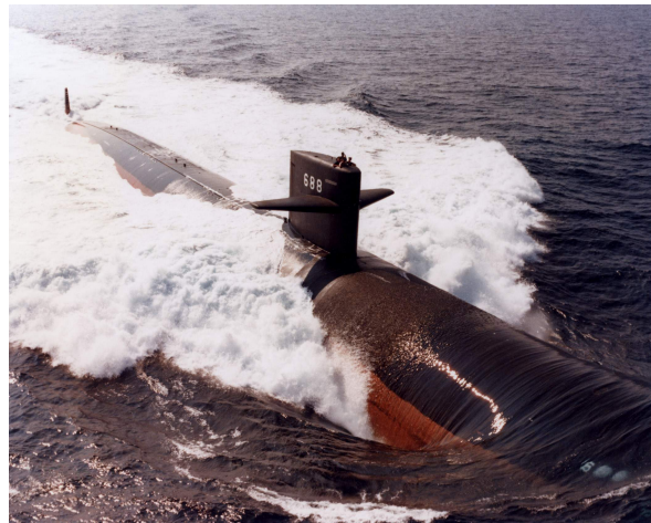
Figure 4.5: Laminar-to-turbulent transition over a submarine hull (image taken from the NavSource Naval History website).
