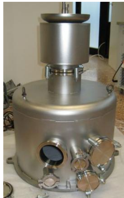
Fig. 7-20 Bottom part and top cap of the TVC for STC-VIHI
