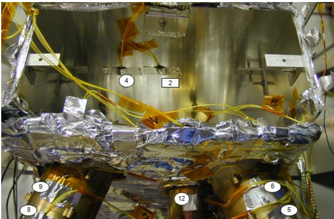
Fig. 4-13 Position of temperature sensors on STC – VIHI unit
