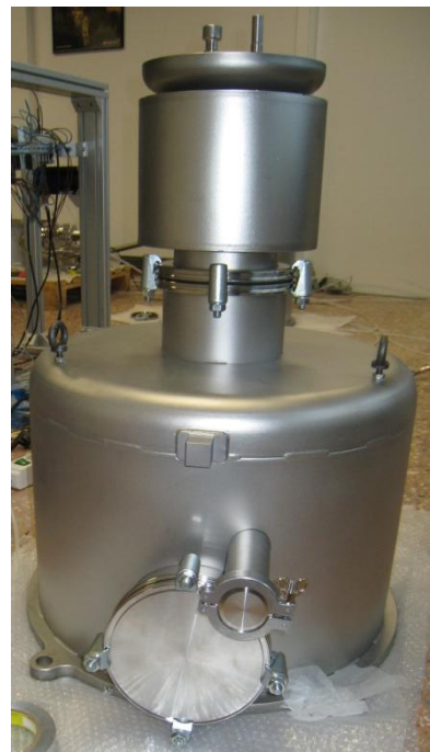
Fig. 7-48 Bottom part and top cap of the TVC for HRIC
