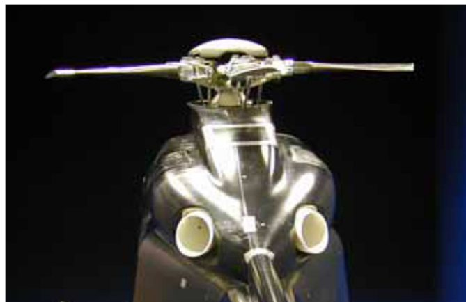
Figure 3.5: AW139 large-scale beanie on the rotating test rig.
