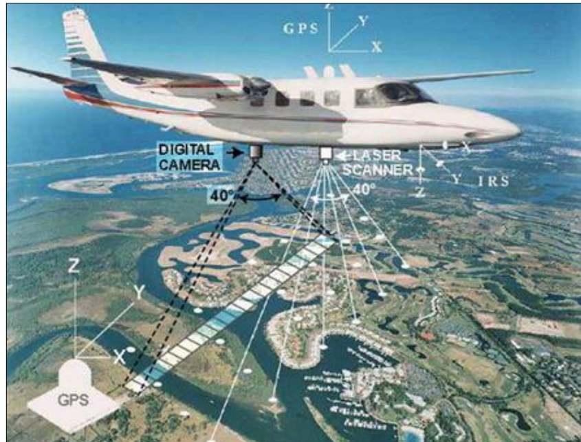
Figure 26: Airborne LiDAR survey technology.
