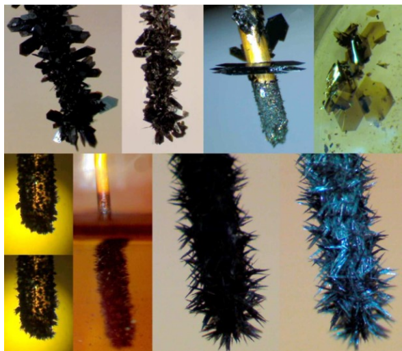
Figure 1.4. Different shapes of crystals of \text{Au}_{25}(\text{SC5})_{18}^0 , \text{Au}_{25}(\text{SC4})_{18}^0 , and \text{Au}_{25}(\text{SC2Ph})_{18}^0 nanoclusters covering the electrode surface, as prepared by the electrocrystallization strategy. (From ref. 102)
