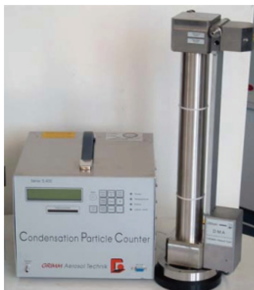
Figure A4.4. Scanning Mobility Particle Sizer (SMPS+C, Grimm Aerosol Technik®)
