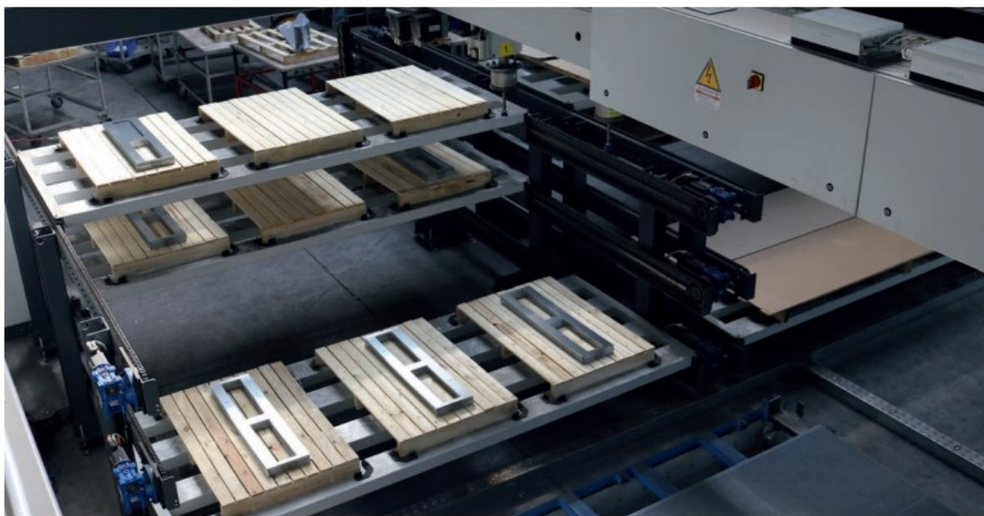
Figure 49 - Automatically sorting plates of steel inside Company E
