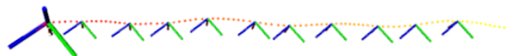
Figure 5.4: Trajectory and keyframes during a forward camera motion. The full trajectory is represented by colored dots while selected keyframes are represented as frames. The blue axis is the camera z axis, or the view line.
