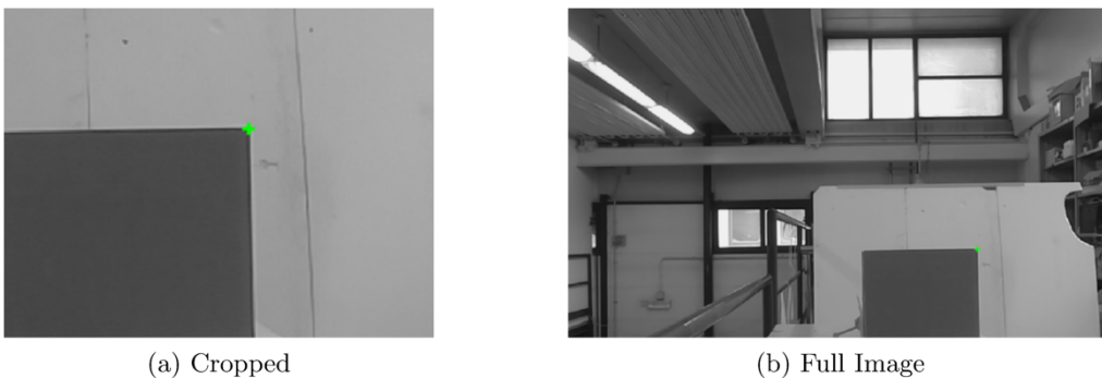
Figure 4.7: Example of plate corner detection on a camera frame. (a) cropped to the interest region, (b) full image undistorted. The green cross identifies the highest scoring Harris corner.
