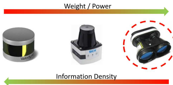
Figure 5.1: Simple overview of range sensor types. From left to right, 3D sensors such as the Velodyne Puck family provide the highest information content at the price of a higher weight and power required. In the middle, 2D LiDARs such as the SICK LMS family represent a compromise between mass and power budget while on the right, LiDAR altimeters provide the lowest amount of information possible as well as being lightweight and inexpensive.
