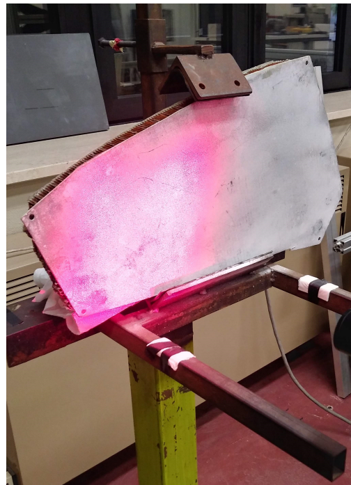
(b) Sandwich panel composed by a honeycomb core and fiberglass skin.
