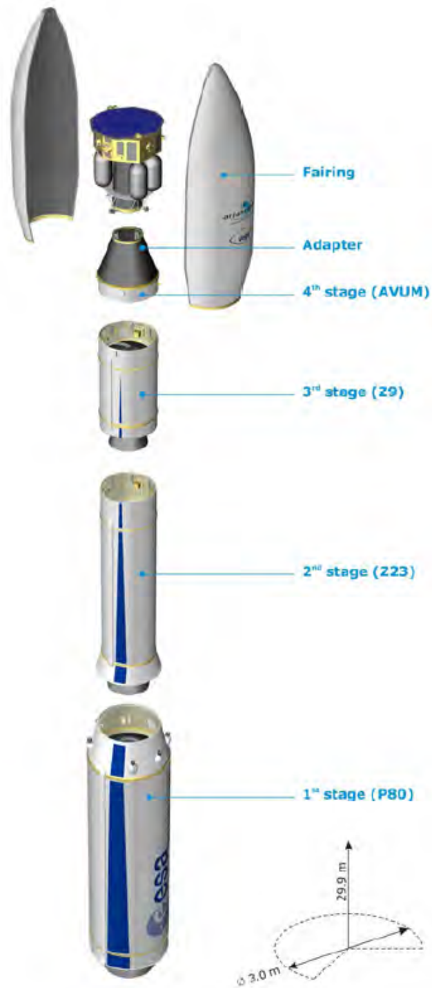
Figure 1.2: Principal stages of Vega launcher. Composite parts are: upper stage, inter-stage section, fairing and adapter.
