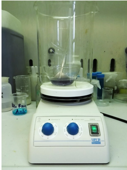
Figure 2-13. Immersion of the component in the acid solution. The magnetic plate assures the mixing and the heating.
