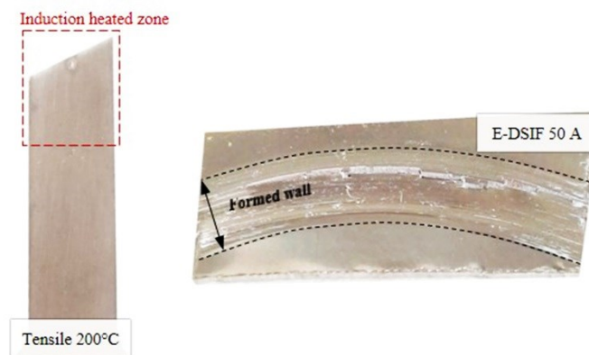
Figure 6-18. Qualitative chromatic comparison between the samples obtained from the tensile and E-DSIF tests performed at 200°C and 50 A, respectively. The red box represents the area heated by the induction system during the tensile tests.
