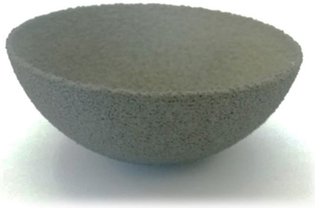
Figure 1-2. Ti6Al4V shell characterized by a high surface-to-thickness ratio [courtesy of Eurocoating].
