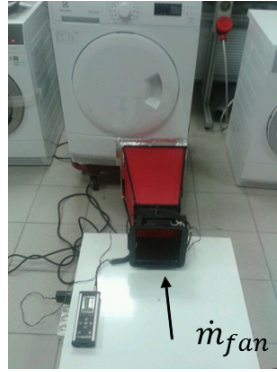
FIGURE 3.5: Measurement of the cooling fan mass flow rate.
