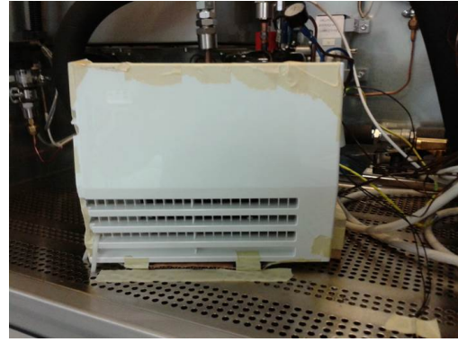
FIGURE 2.40: Compressor measurements with cooling fan in a calorimetry rig.
