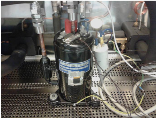
FIGURE 2.39: Compressor measurements in a calorimetry rig.
