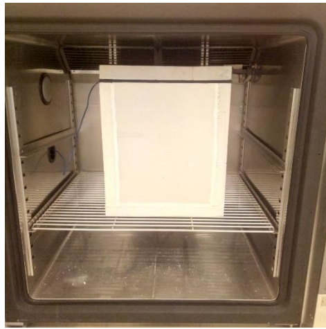
Figure 5.6.6 Cubic test cells developed to assess the thermal responsiveness of different IP mortars.
