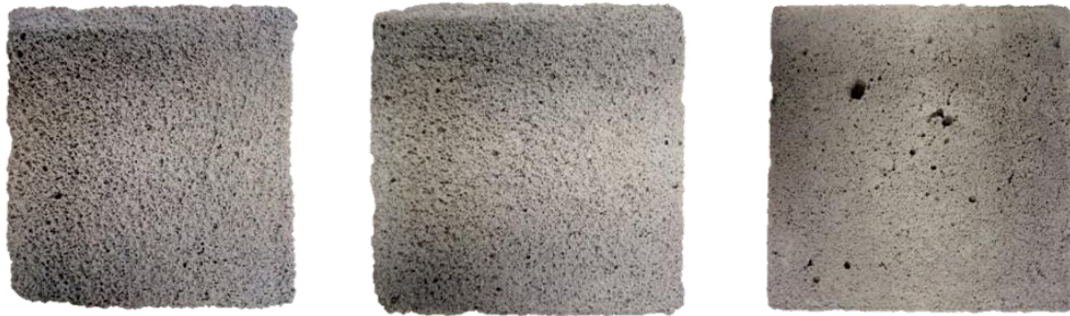
Figure 4.5.7 Image of porous IPs produced using precursors with different particle size distribution (Blaine value growing from left to right).
