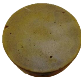
Figure 4.5.19 Lightweight alkali-activated materials produced with hollow glass spheres.
