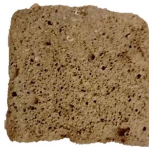
Figure 4.5.2 Illustrative image of porous IPs produced using pre-foaming methods.
