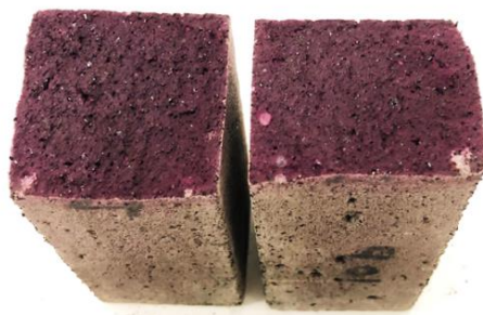
Figure 5.6.4 Illustrative image of the lack of carbonation in PCM-coating samples at time 0.
