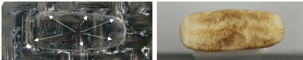
Figure 2.77 Analysis of the interface in the process induced riveting
