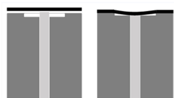
Figure 2.75 Example of process-induced riveting after having removed the aluminum insert
