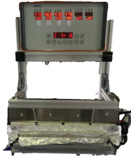
Figure 2.28 Heating system for melting of the external area of the stems
