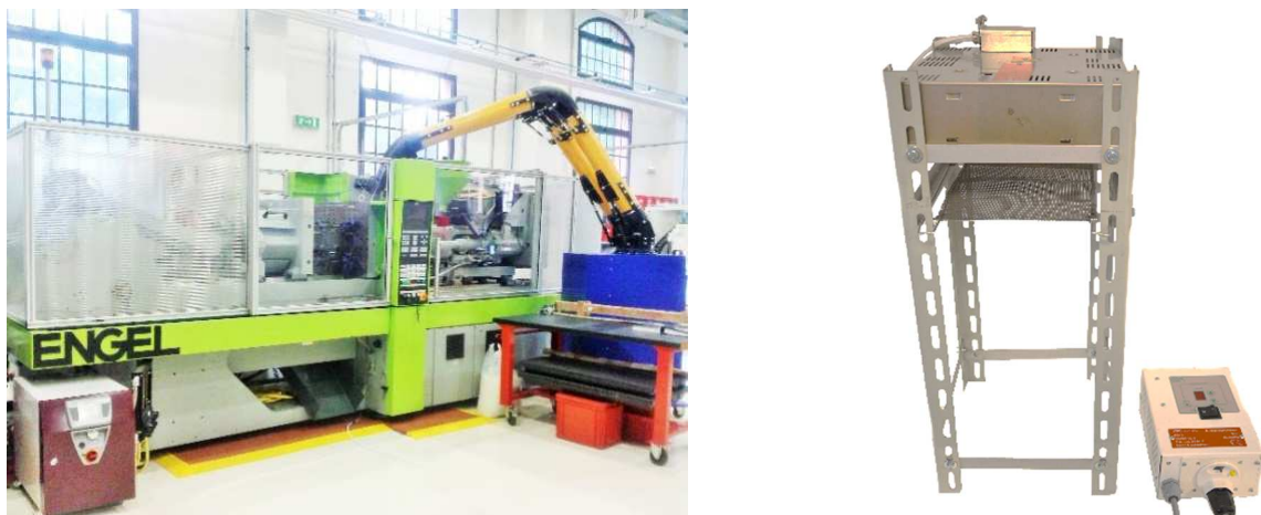
Figure 2.22 Machine and devices used for the manufacturing of the hybrid T-joint specimens
