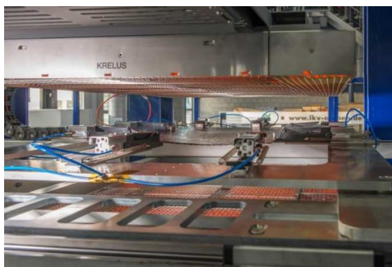
Figure 2.27 Rectangular frame with pneumatic clamps and detail of a single clamp
