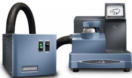
Figure 2.12 Differential scanning calorimeter DQ200 (TA Instrument)
