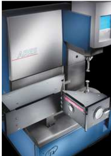
Figure 2.9 Rotational Rheometer ARES G2
