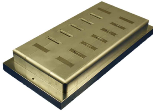
Figure 2.25 Supporting system for the stems with 14 slots
