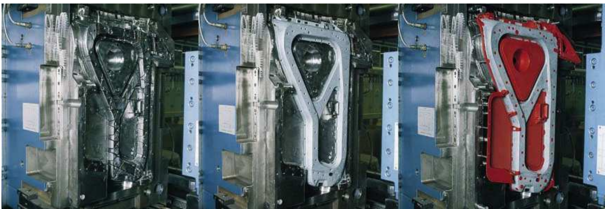
Figure 1.3 Process steps for the manufacturing of an automotive part in metal/polymer composites [59]
