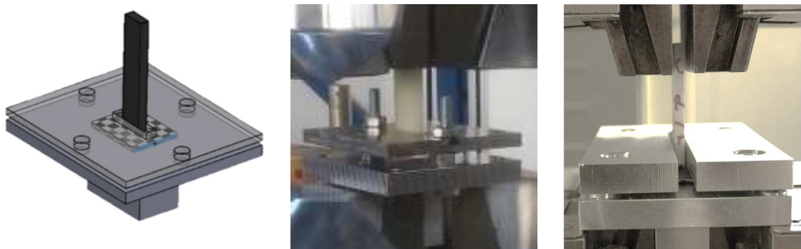
Figure 2.32 Clamping systems for the base of the specimen that were used during the tensile test
