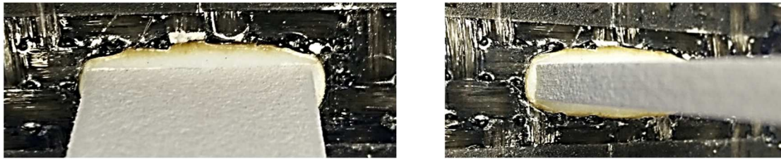
Figure 2.76 First experimental trial with process induce riveting
