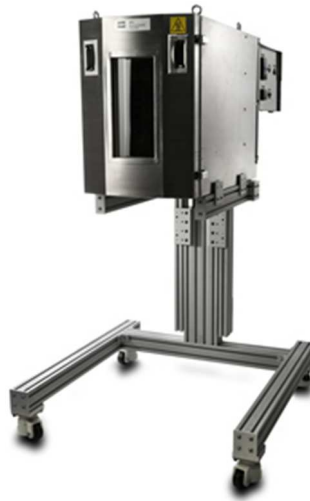
Figure 2.24 MTS environmental chamber used for the annealing treatment
