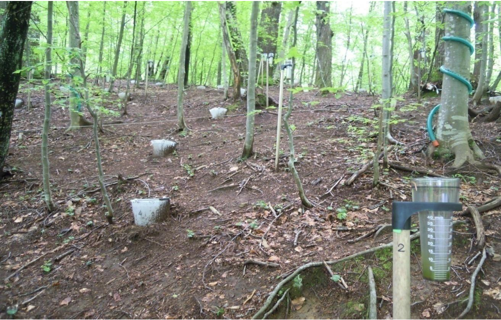
Fig. 3.2.4. Buckets and rain gauges installed in the experimental plot.
