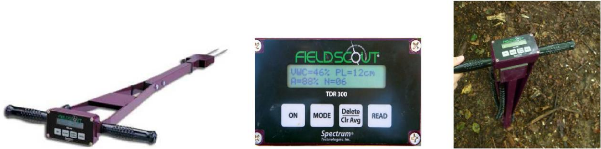
Fig. 3.2.6. TDR probe used for the soil moisture measurements at the throughfall plot.
