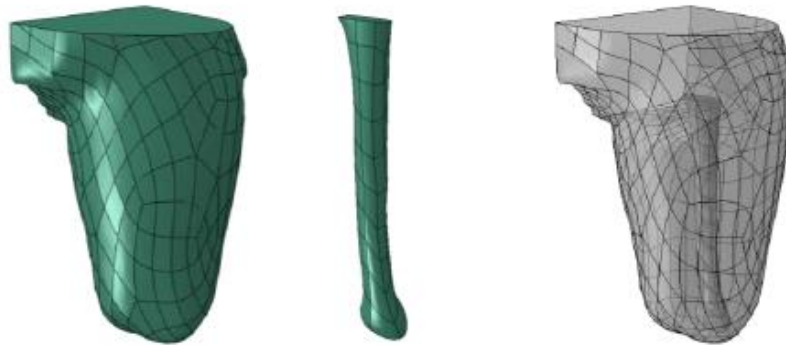
Figure 22: External shape of the residuum and internal bone automatically reconstructed by MRI volume.
