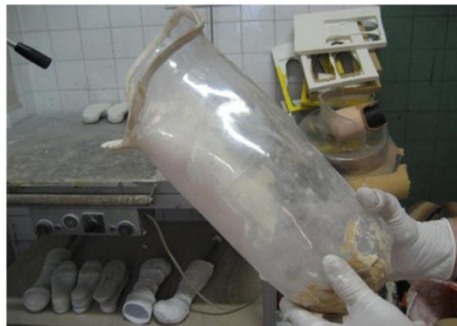
Figure 5: Thermoformed socket of a socket for above knee amputation.
