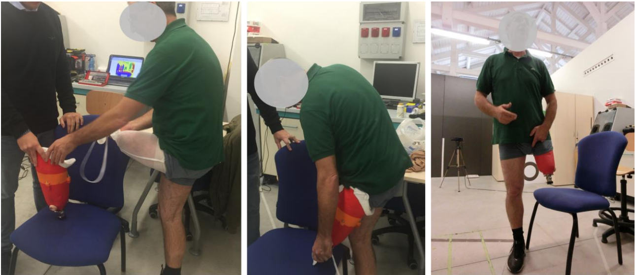
Figure 80: Donning of the 3D printed socket.
