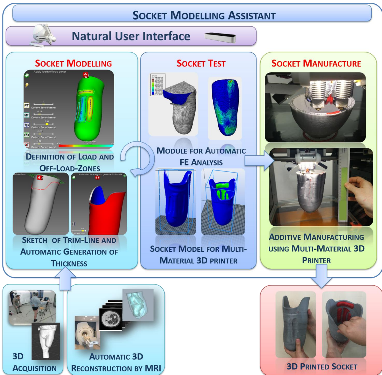
Figure 16: SMA 2 high-level architecture.
