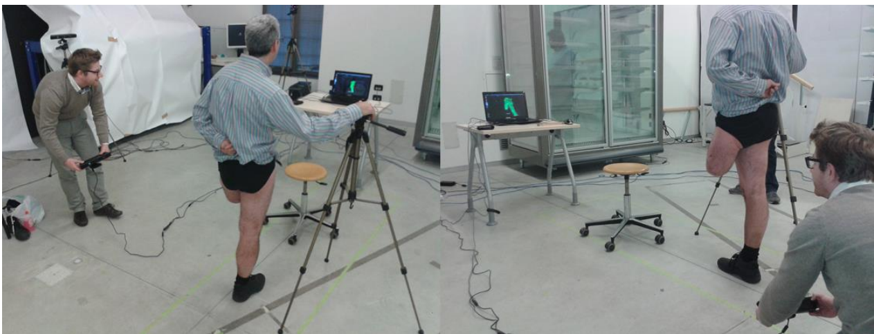
Figure 46: 3D scanning procedure of a lower limb patient with MS Kinect v1.
