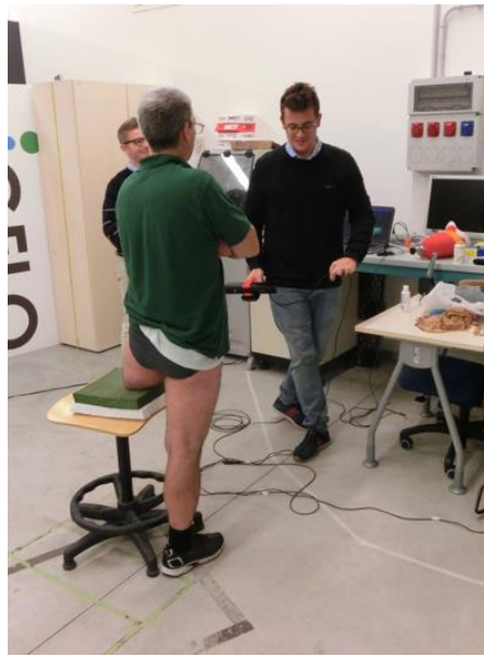
Figure 77: 3D acquisition using Microsoft Kinect v1 and Skanect and with a stand for residual limb.
