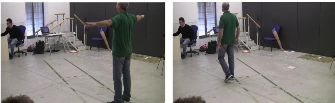
Figure 82: Gait acquisition with iPiSoft system.
