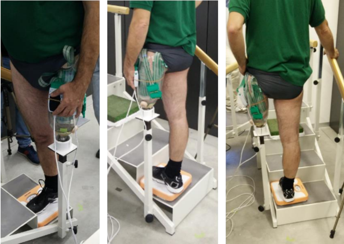
Figure 85: Static test of pressure acquisition.
