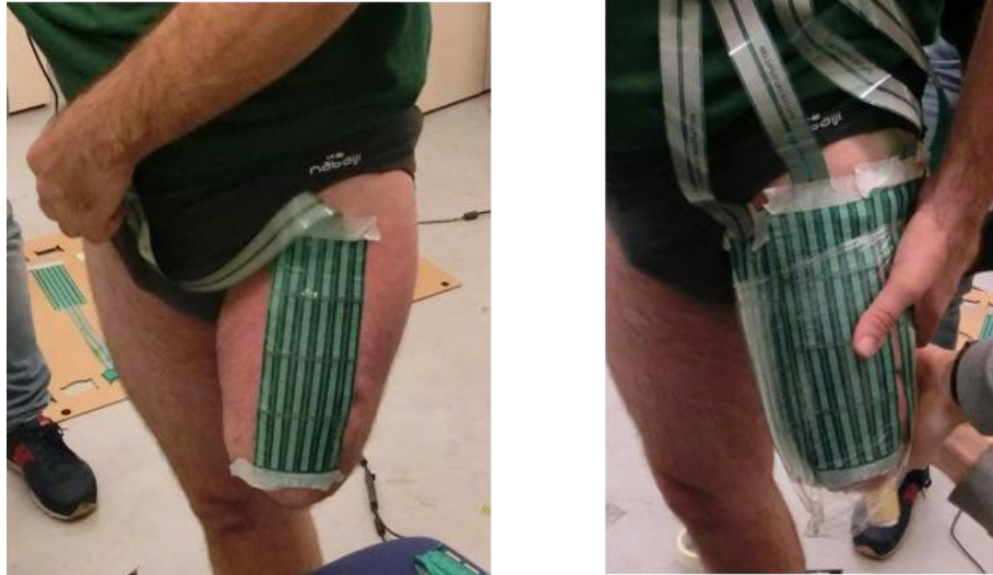
Figure 84: Tekscan sensors applied on the residual lower limb.
