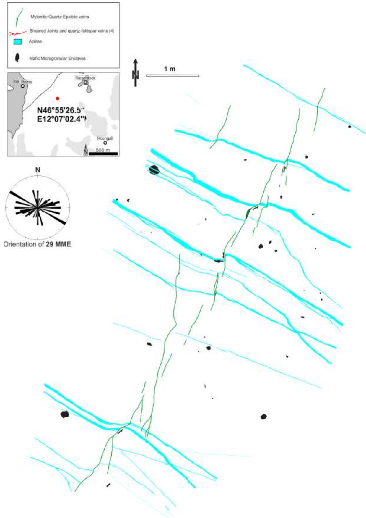
Figure Supplementary Material 3: Surface map of the studied outcrop WP039. Structures that can be identified here: aplite-pegmatite dykes, Stage 2 en-echelon mylonitic veins. The orientation of the elongation of mafic enclaves is reported in the rose diagram.
