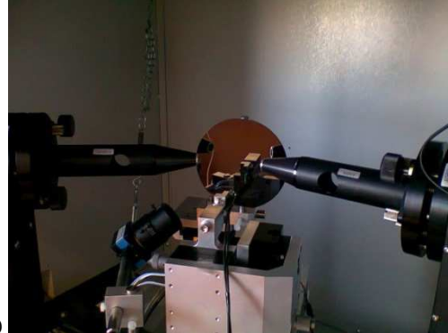
Figure 6.6 Final EllipsSNOM setup. (a) Overall picture; (b) SNOM head and sample holder; (c) The whole system during a routine calibration scan of the ellipsometer, with the focusing probes mounted.
